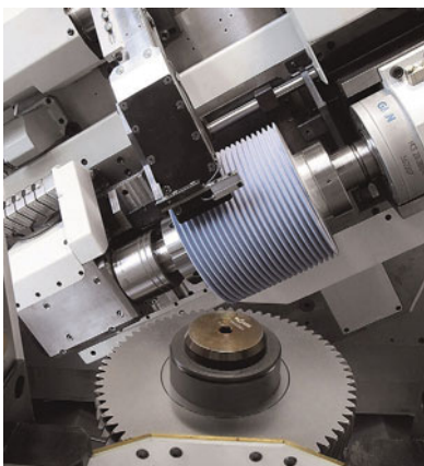
The high-speed grinding element of the G 250 HS makes it possible to grind workpieces with interfering contours using small generating and profile grinding wheels.
